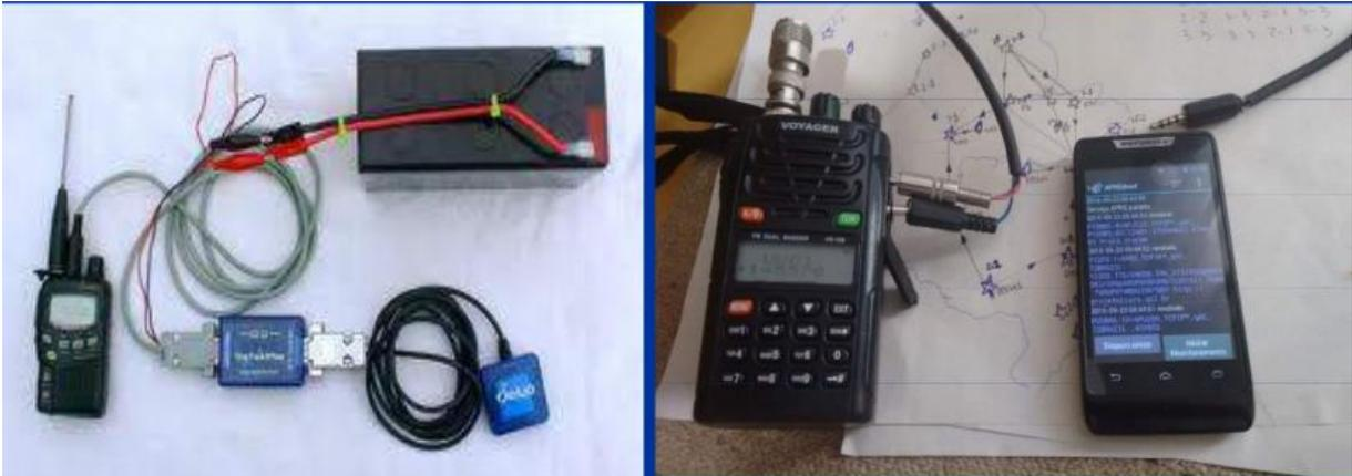
**Figura 8:** *Tracker com TNC e Tracker com smartphone*
